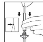
Hold catheter and pull down strain relief tube
