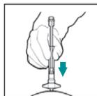
Slide strain relief sheath down and attach to compression cap
