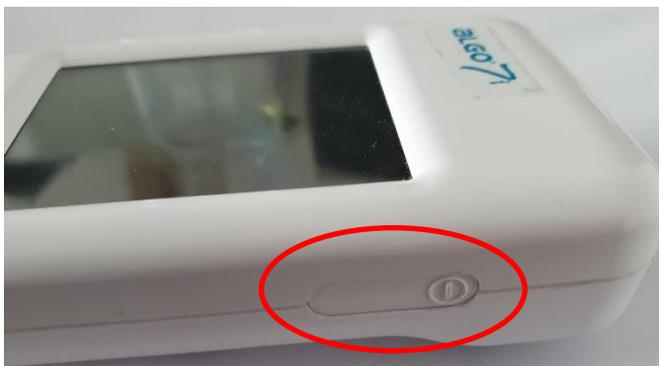
*Figure 2: On/off switch*
