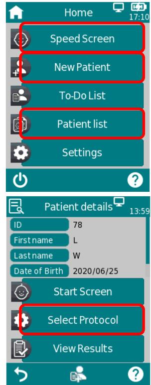
If you want to start screening immediately and enter Patient data during screening, touch “Speed Screen”. You will be directed to the Screening display and measurement will automatically start, if ATA Cable and Patient Cable are connected properly to the device. You can then enter the patient’s data by tapping on the individual field using the touch screen display.
