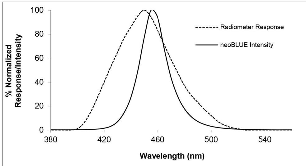
The light output was factory calibrated with the neoBLUE Radiometer to provide an initial intensity of  $35 \mu\text{W}/\text{cm}^2/\text{nm}$  at the high setting and  $15 \mu\text{W}/\text{cm}^2/\text{nm}$  at the low setting at a distance of 12 inches (30.5 cm) from the light enclosure to the baby. This measurement is taken at the central area of the effective surface area for phototherapy.
