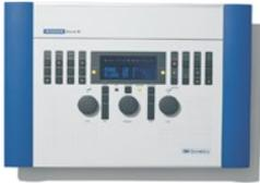
MADSEN Itera II is an audiometer for testing a person's hearing.
