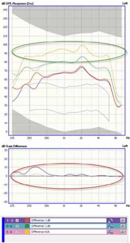
The comparison of measurements is made by viewing the dB Gain Difference curves (55 and 80 dB measurements – red oval) and the dB SPL Response (MPO – green oval).
