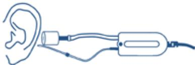
*Note: This insertion depth means that the tip of the probe tube is likely to be within 5 to 6 mm of the tympanic membrane. Otosuite contains a user test designed to assist with proper probe tube placement via acoustical positioning procedures described in ANSI, 1997 and in ISO 12124:2001. A simplified method is through visualization and repositioning based on the REUG curve, monitoring particularly the frequency region above 4000 Hz.*
