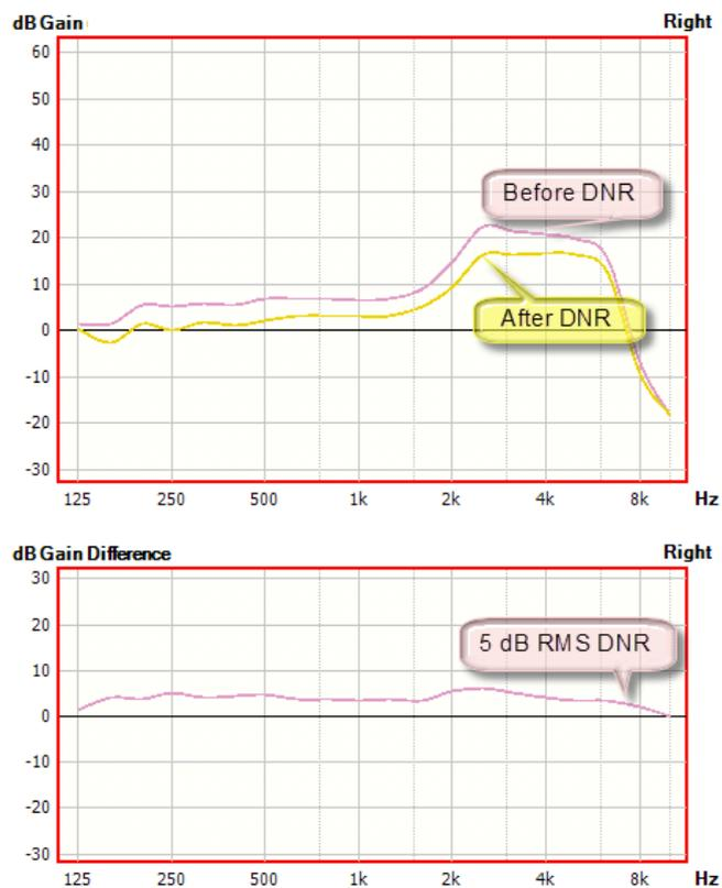
**Figure 6.** DNR measurement curves. The pink curve in the top graph is the short term average (STA) curve taken before DNR is activated. The yellow curve is the STA taken after DNR engaged. There is a noise reduction of 5 dB RMS observed.
