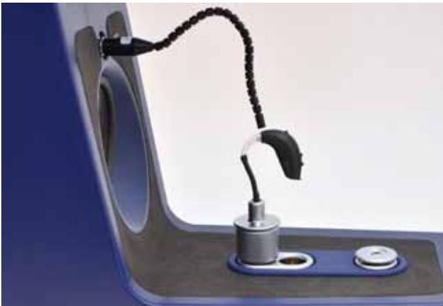
Figure 2: Positioning of the hearing instrument and reference microphone in AURICAL HIT.
