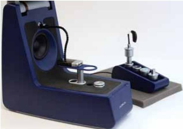
Figure 5: Positioning of the hearing instrument outside AURICAL HIT in the external accessory module. The Mini Microphone is positioned on the elevation plate in AURICAL HIT.
