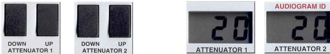
Normally the steps are 5 dB, but by means of the 1 dB button the steps can be changed to 1 dB. Held down for a while, the attenuators will repeat.
