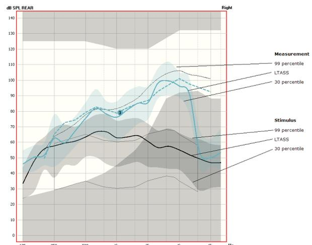
Further, it is possible to compare the measured speech spectrum with that of the known stimulus input spectrum to see the impact of the amplification on the dynamics of speech.
