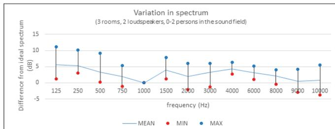
Fig. 1 The variation of the signal spectrum measured acoustically in 3 rooms, using 2 different loudspeakers and with 0, 1 and 2 persons in the room. All curves were normalized at 1 kHz.
