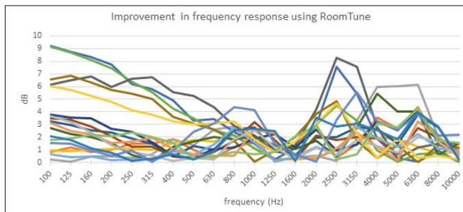
Fig. 2 The graph shows how many dB RoomTune improved the accuracy of the presented signal in 3 different rooms using 4 different speaker systems (3 stereo and 1 mono).
