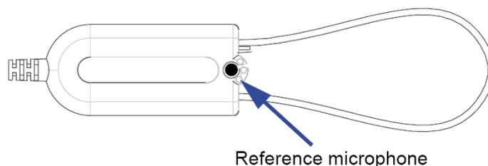
Figure 1: The reference microphone on the probe is located at the ear of the subject during measurements.
