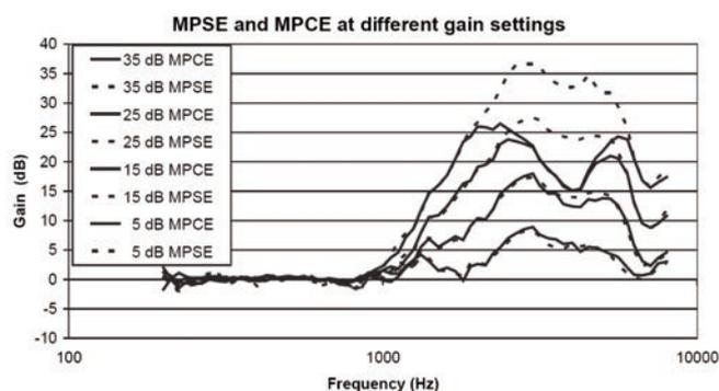
Figure 2: The REIG measured with MPSE and MPCE methods with four different gain settings in a single subject. The measuring error increases as a function of the digital feedback suppression benefit (from Lantz et al.).
