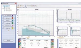
Clicking the Historical Data icon will bring up a window with previously collected data. Check one or more of the boxes and you will see the results and probe fit information overlapped as well as the data table for numeric comparisons. Highlighting a box will show the numeric information in the data table. The other curves will be represented by a thin line with no symbols.
