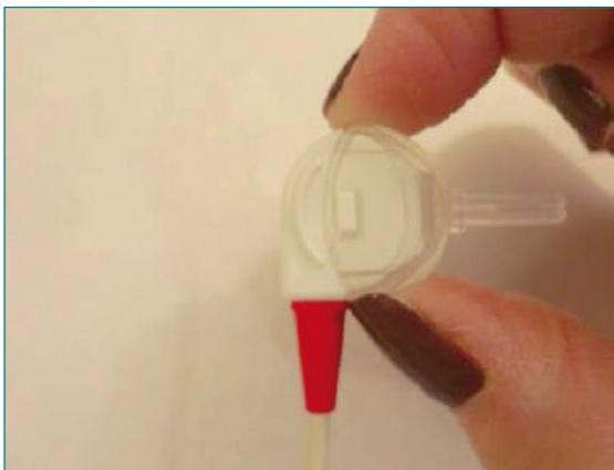
If you continue to receive a probe failed result, please make sure that all of your connections are secure. Also, try removing the clear plastic probe tip by gently squeezing the top and bottom of the tip. Continue squeezing as shown and hold the probe body (white part just above the red), pull gently to remove. Rotate the tip 180 degrees and place the tip on the probe. Repeat the probe test.
