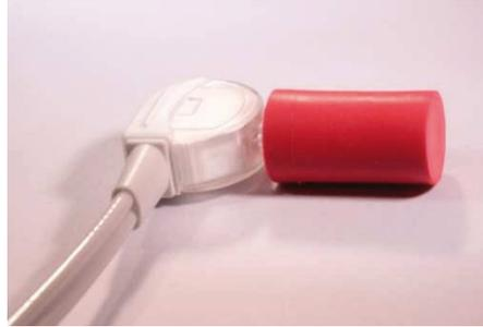
When probe is sealed, tap the pump unit test button:
