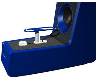
Use the elevation plate to facilitate positioning of wireless transmitters and body worn hearing instruments at a level where the microphone or microphones are approximately centered in relation to the loudspeaker.
