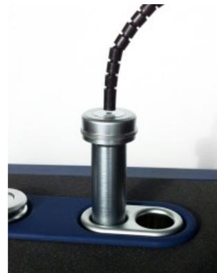
3. Position the reference microphone (1) pointing straight down from above and centered 1-2 millimeters above the coupler measurement microphone (3).
