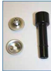
The E2E verification kit includes a passive coupler and 2 coupler adaptors allowing you to place the transmitter device inside AURICAL HIT just as a normal hearing instrument. The receiver device is attached to the regular coupler and placed in the external accessory module connected to AURICAL HIT.
