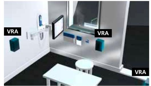
The optional paediatric test modality in OTOSuite® for the MADSEN Astera<sup>2</sup> audiometer is compatible with the animated Visual Reinforcement Audiometry (VRA) solution from Pehrtek. The professional has full control over both the sound stimulation and the visual reward for the child, either through the Audiometer Control Panel, via the PC or an infrared transmitter. The solution consists of the modules below:
