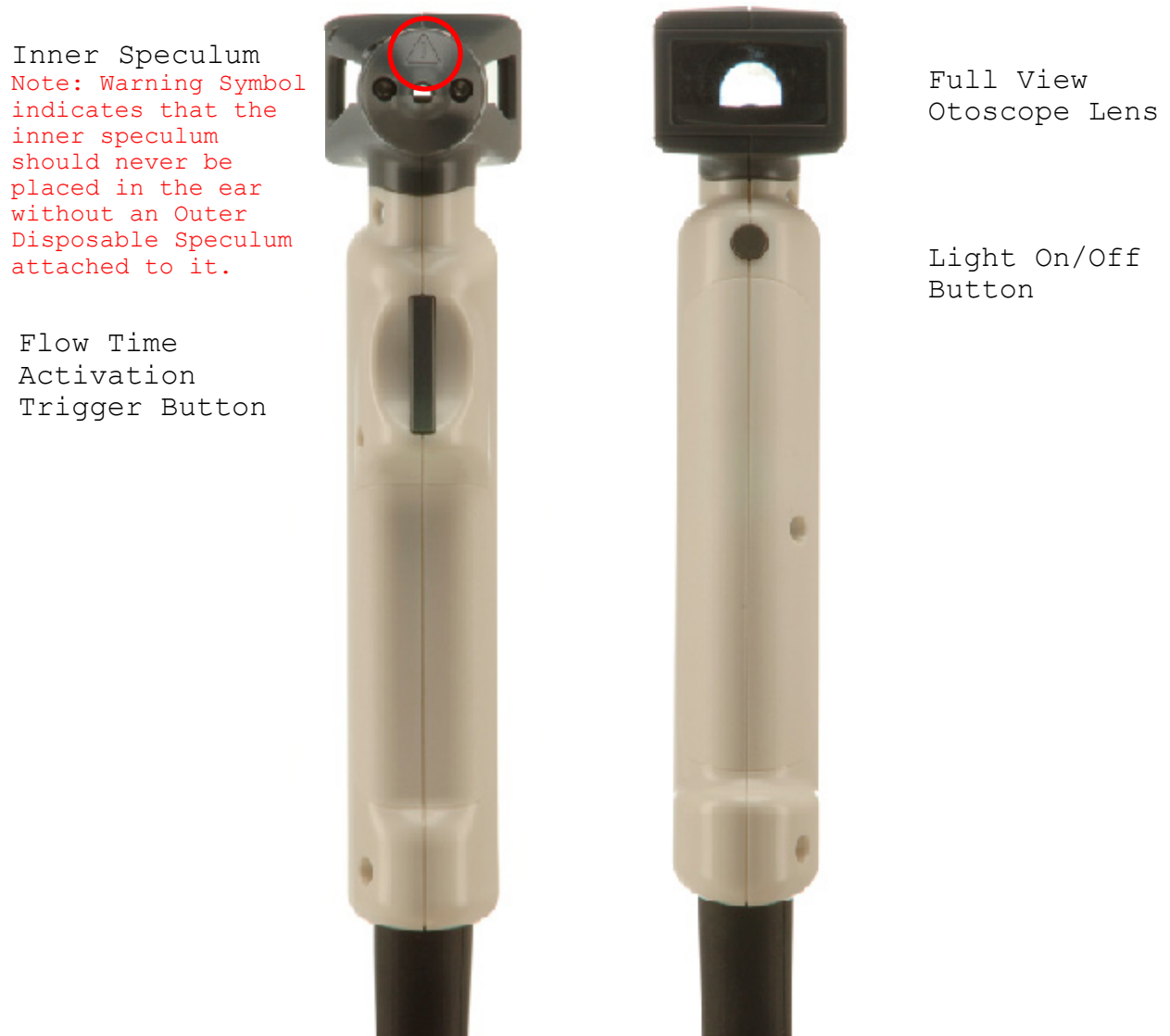
Figure 4: Front and Back views of the NCA-200A delivery head and controls.
